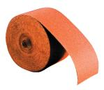
VC-152 Medium 115mm x 50m Rolls. Stable aluminium oxide abrasive paper for universal use. Low loading characteristics. Flexible paper backing. Used for manual and mechanical sanding on metal, wood, lacquer, paint, primer, filler, plastic and aluminum.
