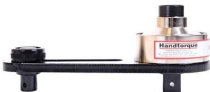
Multiple stages of epicyclic gearing are used in Norbar's 'HandTorque' multipliers to provide a wide range of torque outputs and ratios to suit most applications. The torque multiplication ratio is always quoted, not the velocity ratio as some competitors' goods claim. For example, a velocity ratio of 29.8:1 would result in a torque multiplication of 25:14%.
