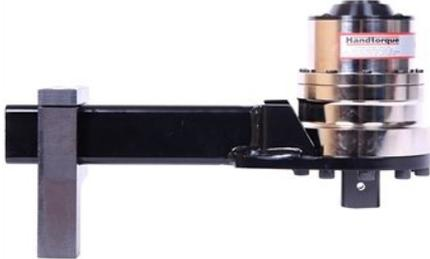
Multiple stages of epicyclic gearing are used in Norbar's 'HandTorque' multipliers to provide a wide range of torque outputs and ratios to suit most applications. The torque multiplication ratio is always quoted, not the velocity ratio as some competitors' goods claim. For example, a velocity ratio of 29.8:1 would result in a torque multiplication of 25:14%.
