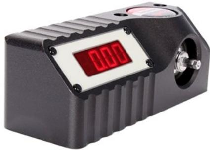
This TruCheck torque tester is ideal for checking Torque Screwdrivers and small Torque Wrenches. It comes with a single measurement unit, Ni $\frac{1}{2}$ m. There is only one button on the device and that is to zero the display. Operation is simplicity itself and it is virtually impossible to go wrong! TruCheck 25 Ni $\frac{1}{2}$ m has an accuracy of  $\pm 1\%$ ,  $\pm 1$  digit over the stated operating range and comes with a traceable calibration certificate. Range: 1 - 25 Ni $\frac{1}{2}$ m
