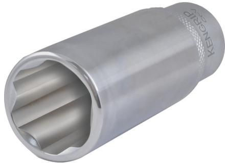
3/8 Square Drive Conform to DIN3124. The Ken-Grip® socket offers a new standard of performance with the ability to grip up to 95% of a rounded fastener. Double knurl feature gives a high grip which is essential for quick tool change when hands are greasy or oily. Manufactured from chrome vanadium steel, the sockets and accessories are aluminium free and fully chrome plated for an easy clean finish
