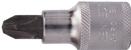
For insertion and removal of fasteners and fixings using 1/2" square drive tooling. Made from chrome vanadium steel, fully chrome plated with a mirror finish and aluminium-free to ensure non sparking. All have ball retaining groove on each face of the square drive. Conform to DIN standards.
