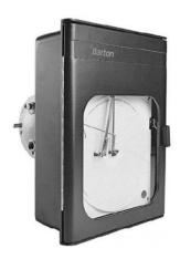
Barton 242E/100°C/15000 Psi/Mechanical | Two Pen Pressure Temperature Recorder | Model 242E | Pressure Range: 0-15000 Psi | Mechanical Chart Drive: 24 HRs/7 Days
