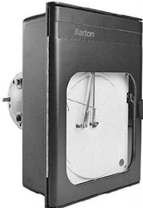
**Barton 242E/2000 Psi/Mechanical | Single Pen Pressure Recorder | Model 242E | Pressure Range: 0-2000 Psi | Mechanical Chart Drive: 2 HR/ 8 HR**
