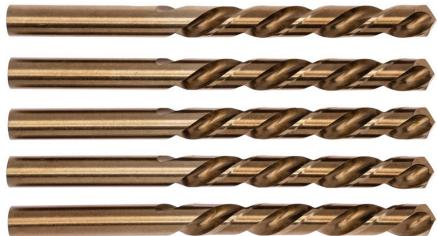
Due to the inclusion of 5% cobalt to their alloys, the Kennedy line of heavy duty straight shank jobber drills with HSS-Co delivers dependable and long-lasting cutting performance at high temperatures and speeds. They can drill steels with tensile strengths of up to 1,400 N/mm<sup>2</sup>, very hard bronze, stainless steels, as well as steels that are heat- and acid-resistant thanks to their toughness and heat resistance.
