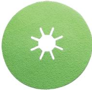
Siabite 4515 High performance sanding disc with ceramic aluminium oxide abrasive type. For use on high-alloy materials including stainless steel, titanium alloys, copper alloys, brass and bronze. Active grinding additives guarantee cool grinding with virtually no discolouration of workpieces and maximum material removal in the shortest time. Diameter: 115mm. Bore: 22mm.
