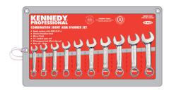
Contains: 10, 11, 12, 13, 14, 15, 16, 17, 18 and 19mm. Manufactured from quality chrome vanadium steel with hardened jaws and high polish mirror finish, corrosion-resistant and easy to clean. The jaws and ring are offset at 15° for easier location and application of torque to the fastener. Suitable for use in areas of very restricted access. Conforms to ASME B107.6.
