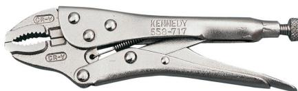
Curved Jaw Specially designed to grip circular objects. Ideal for plumbing and general pipe work. Rolled chrome vanadium steel bodies, drop forged hardened steel jaws with corrosion-resistant bright nickel coating. The jaw opening and clamping pressure can be adjusted with the knurled head screw, fitted with wire spring to ensure efficient opening of the jaws. The locking mechanism holds the wrench in place once adjusted, leaving both hands free.
