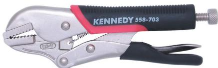
Rolled chrome vanadium steel bodies, drop-forged hardened steel jaws with corrosion-resistant bright nickel coating. The dual material handle design allows the user to apply the greatest force with the minimum amount of effort. The jaw opening and clamping pressure can be adjusted with the knurled head screw, fitted with wire spring to ensure efficient opening of the jaws. The locking mechanism holds the wrench in place once adjusted, leaving both hands free.
