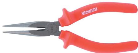
Heavy-Duty Snipe Nose Pliers with Cutter Chrome vanadium steel, heavy-duty handle with slip guard. Double polished head and joint with induction hardened cutting edges. Also with side cutter and serrated gripping and crimping jaws behind the head.
