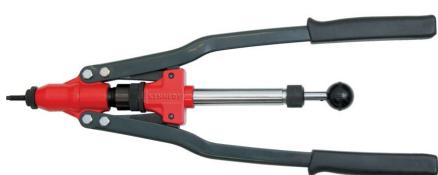
Model RNI410 This sturdy professional quality tool has been designed for the insertion of rivet nuts into sheet metal. It has a cast body with a corrosion-resistant powder-coated finish, heavy-duty steel levers with soft grips for user comfort and a knurled adjustment ring for material thickness setting. It also has a pump action mandrel turning shaft for quick loading of fasteners. Includes: Set of five nose piece kits, M4, 5, 6, 8 & 10 plus instruction manual.
