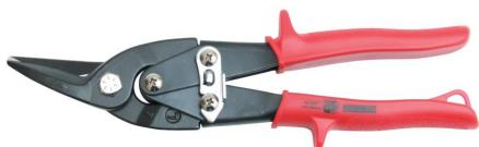
Left Hand or Right Hand Cut Cut from tight curve to straight. Drop forged chrome vanadium ground blades (54 - 58HRc). The double fulcrum compound action amplifies the pressure applied for easier cutting of up to 1.2mm cold rolled steel sheet. Spring loaded, self-opening action for fast, effortless feed and single-handed operation. Anti-slip guards for extra safety. Thumb lock ensures the jaws stay closed when not in use. For use on mild steel and other non-ferrous materials.
