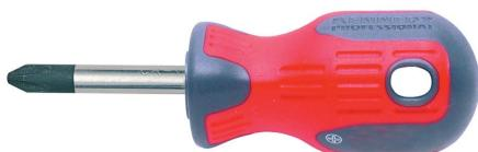
Chrome vanadium steel blades with magnetic tips. Fitted with a unique dual grip triangular handle which has been designed for improved user comfort, allowing more torque to be applied. With convenient hanging hole in the handle for storage. Crosspoint Crosspoint screws virtually eliminate the screwdriver slippage if the correct size is used. The No.2 screwdriver would be suitable for most applications. DIN ISO 8764.
