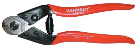
Contoured steel handles with vinyl grip for improved comfort and control. Heavy-duty blades manufactured from tempered and hardened high carbon steel with polished finish. Spring-loaded cutting action for easy one-handed operation with safety lock to keep jaws closed when not in use. Wire rope capacity: 4.8mm, Spring wire: 1.5mm.
