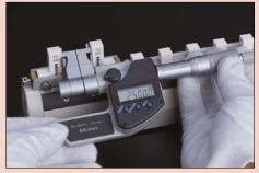
Using an Inside Micro Checker to accurately set an inside micrometer.
