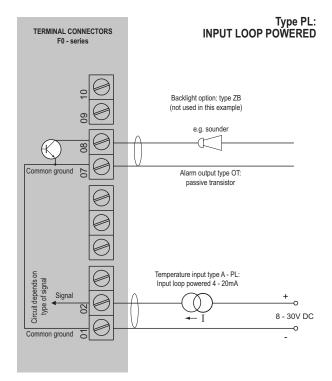
Sensor supply: sensor is externally powered.
