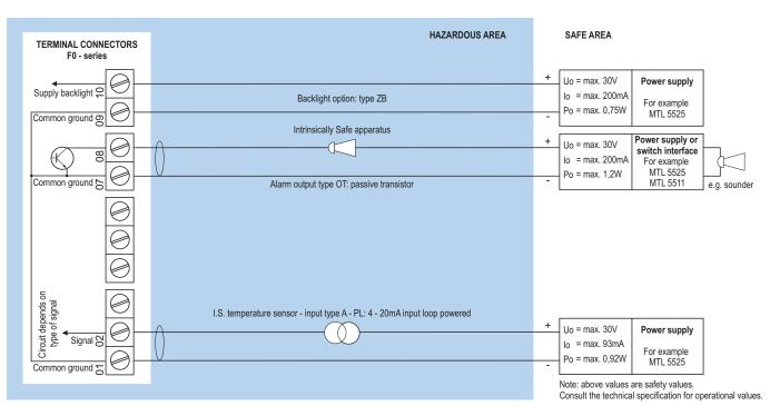
Sensor supply is not available: unit is input loop powered (type PL).
