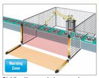
Dividing the zone between seriesconnected sensors
