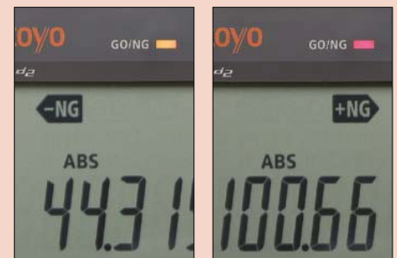
±NG shown on the display and the panel LED showing ORANGE (-NG) or RED (+NG) means the measurement is outside the tolerance limits.
