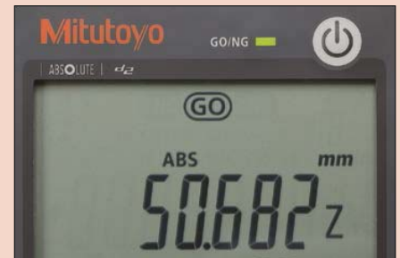
GO shown on the display and the panel LED showing GREEN means the measurement is within the tolerance limits.
