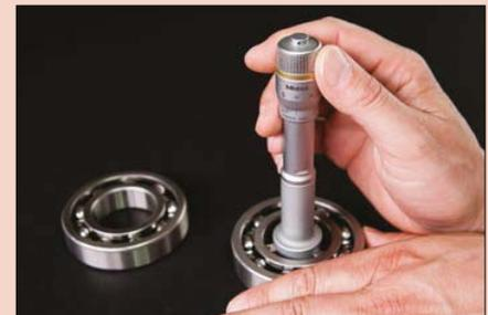
Ball-bearing inner-race inside diameter measurement.
