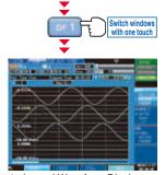
4-channel Waveform Display Display the voltage and current waveforms on channels 1 to 4 individually.
