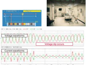
Voltage and Current Waveforms at the Time Voltage Dip Occurs
