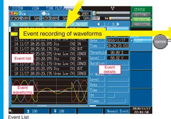
This list records instantaneous waveforms of power supply failures
