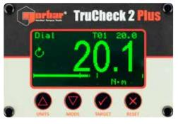
TruCheck™ 2 Plus display showing within target tolerance
