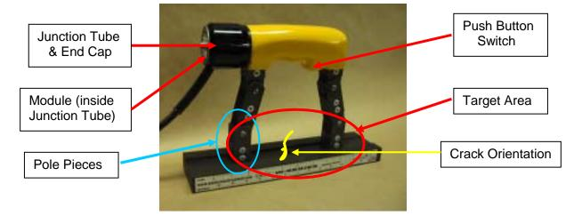
1. Solid State Push Button Switch – The Solid State Push Button Switch was designed for comfort and safety. While depressed, the switch delivers a ½ Watt control signal to the electronic controls (semiconductors) sealed in the Output Module. The Module connected to a receptacle plug in the Junction Tube of the Yoke, and supplies the necessary power (AC) to the coil encapsulated in the Yoke housing.
