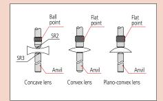
Lens thickness measurement application examples. Note: Parallelism between the flat point and anvil is 10  $\mu m$ .
